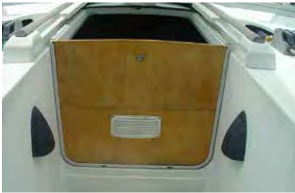
Washboards Boards used to seal off the companionway to prevent the entry of water.
