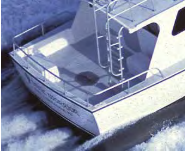
Cockpit A self draining recess in the after part of a vessel.
