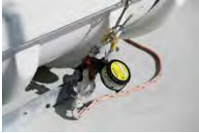
Hydrostatic Release attached to the liferaft
