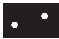
> than 50 m, side, starboard
